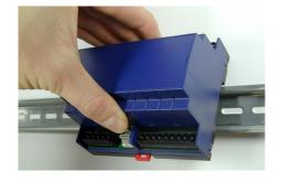
First, place the upper guide edge of the module on the top-hat rail.
