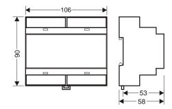
The device has been designed for DIN rail mounting. The housing is a standard size and is also suitable for installation in fuse boxes, distribution switch boxes or electric boxes of refrigerators.
