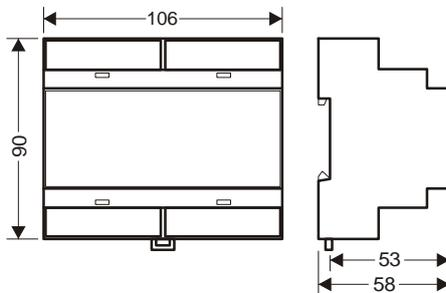
This device is designed for top-hat rail installation. The housing is of a standard size and is also suitable for installation in fuse boxes, distribution switch boxes or electric boxes of refrigeration units.
