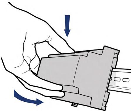
Place the device with the upper guide edge on the top-hat rail.
