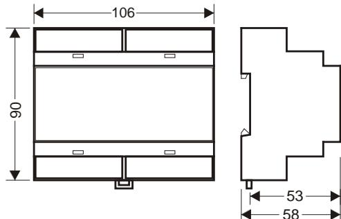
This device is designed for top-hat rail installation. The housing is a standard size and is also suitable for installation in fuse boxes. The devices can be positioned next to one another without gaps.
