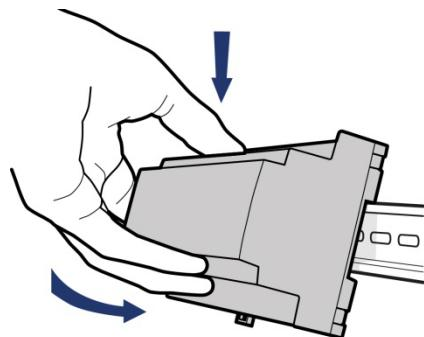
Place the device with the upper guide edge on the top-hat rail.
