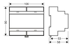
This device is designed for top-hat rail installation. The housing is of a standard size and is also suitable for installation in fuse boxes, distribution switch boxes or electric boxes of refrigeration units.
