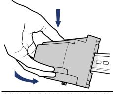
Place the device with the upper guide edge on the top-hat rail.
