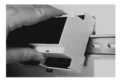
First, place the upper guide edge of the module on the top hat rail and then press it gently downward until it engages with the mounting safety catch on the rail.
