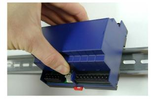
First, place the upper guide edge of the module on the top-hat rail and then press it downwards gently until it engages with the mounting safety catch on the rail.
